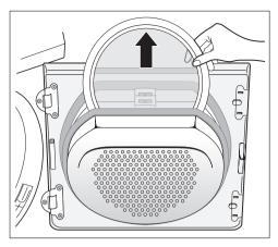
Remove the fluff from fine filter. It is best to use a damp hand for this purpose.
